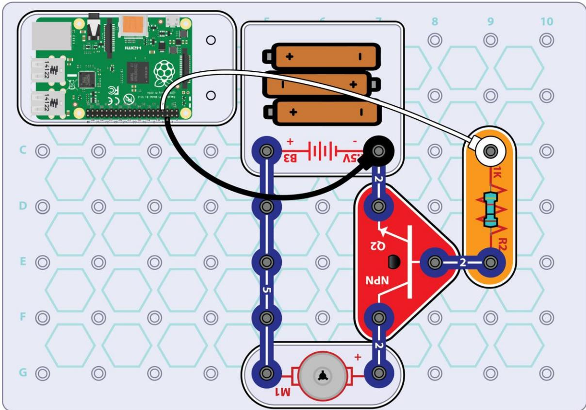
Firstly place the battery plate, motor, R1 and Q2 transistor on the base plate. These will go first as the bridges sit on top. If you would like the fan to spin off the motor, ensure the + marking on the motor is next to the transistor. Link up the components with the 5 snap bridge and the 2 snap bridges.
