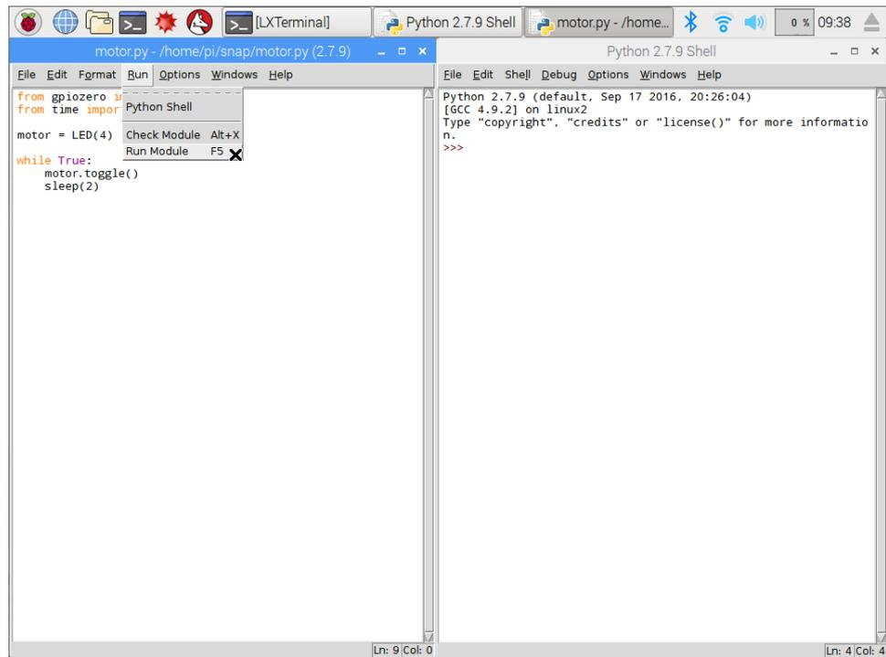
Immediately the motor will start to spin for 2 seconds and then stop for a further 2 seconds before starting again. As this was created with a `while True:` loop, this will run forever until told to stop.
